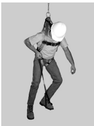
Insert foot into loop step and adjust
