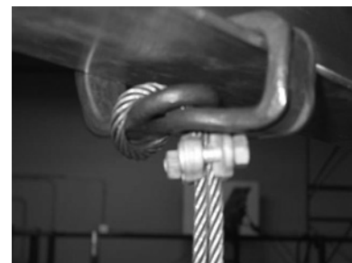
Use fist grips to secure this device during unloading
