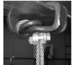
Use fist grips to secure this device during unloading
